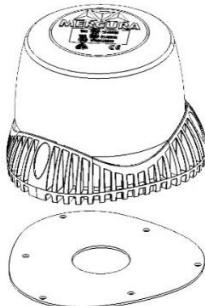
The GYROLED® M130 MERCURA is a CLASS 2 very high-performance LED GYROPHARE. The beacon has 13 integrated operating modes.
